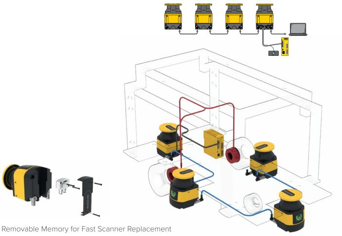
The system configuration is backed up in a removable memory unit. Install your replacement scanner quickly and easily, without needing to reconfigure your system.
