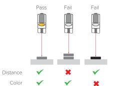
Inspections use distance to verify parts' presence and position, and intensity to verify correct color or part orientation
